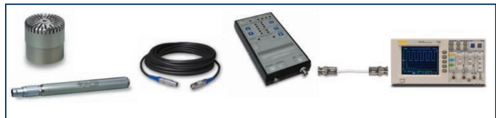
Fig 9. Traditional Externally Polarized set-up
